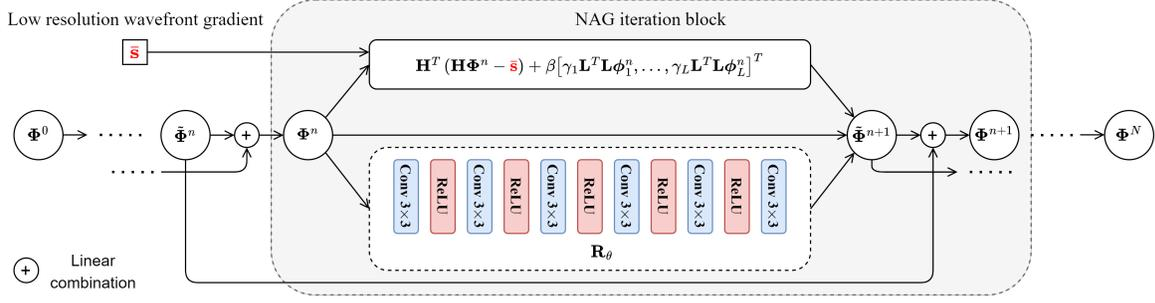
Figure 4: Data flow and network architecture in PhaseNet.
