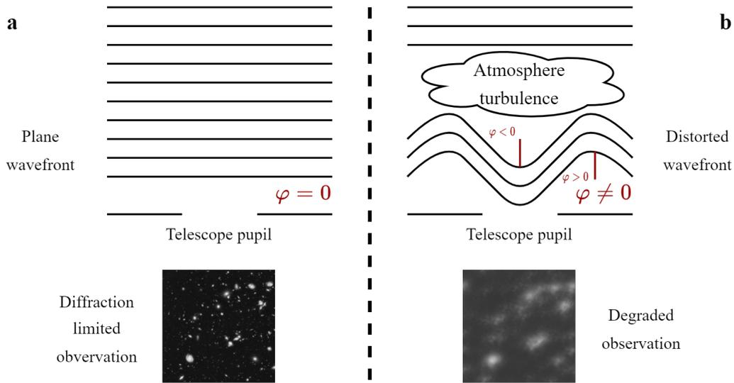
Figure 1: Illustrate the relation between wavefront and phase  $\varphi$ . a: no atmosphere distortion, corresponding to plane wavefront and  $\varphi = 0$ . b: wavefront is distorted by atmosphere turbulence,  $\varphi$  measures the intensity of the distortion.
