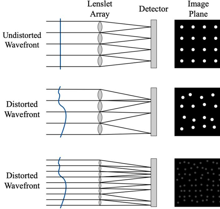
Figure 2: Principle of the Shack-Hartmann wavefront sensor: (top) undistorted wavefront, (middle) wavefront distorted by atmospheric turbulence, (bottom) distorted wavefront with fine-grid lenslet array.
