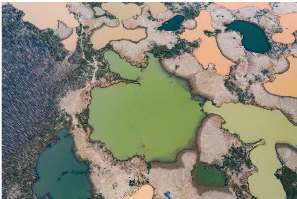
Figure 1: Mining ponds in La Pampa showing a range of activity levels. Deep green ponds indicate the presence of algae and the cessation of mining activity. Chalky clay-colored ponds contain high levels of suspended sediment and are currently actively mixed. Light green ponds, such as the one in the center of the image, are transitioning from active status to inactive status.
